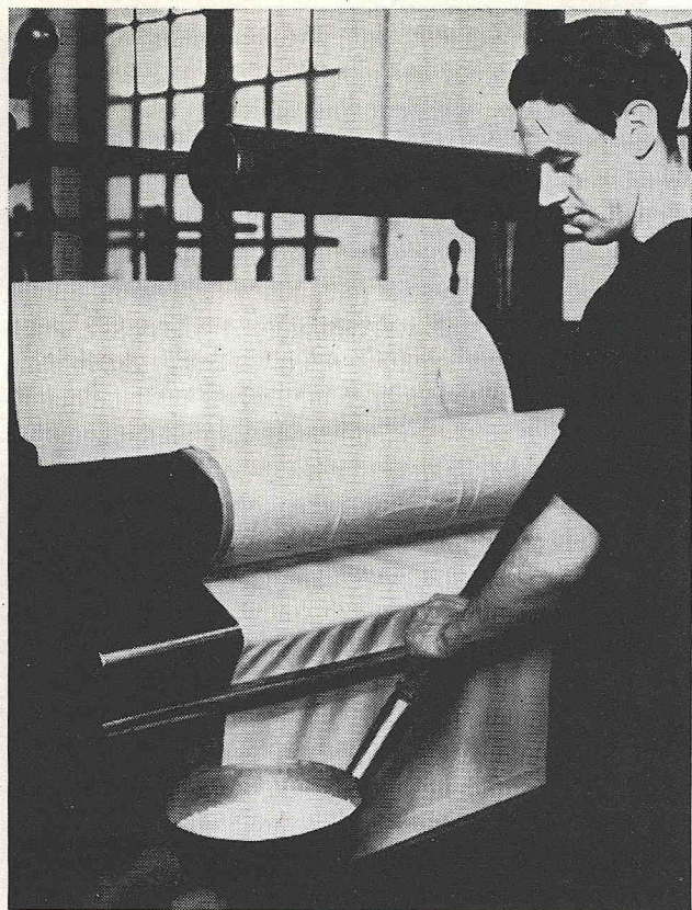
Figure 7. Scouring with Sodium Metasilicate Solution on Jig
